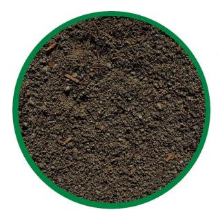
To create this material we blend sand that is specifically designed and manufactured to meet most BMP/LID manual specifications at a rate of 80% by volume sand to 20% by volume high quality greenwaste compost. NO manure or biosolids are used in our line of bioswale growing media.
